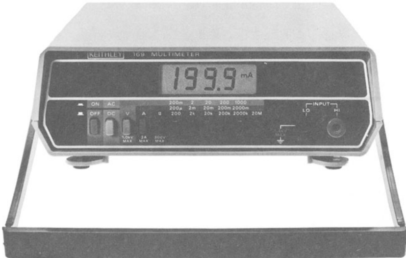
Figure 10.12. Digital multimeters: (a) AVO Model DA116 (courtesy of AVO Ltd), (b) Keithley Model 169 (courtesy of Keithley Instruments Ltd)
