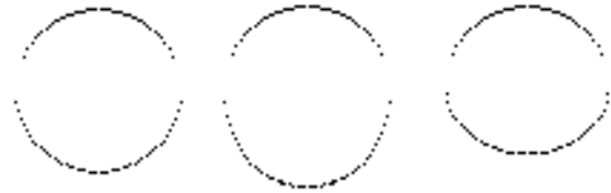
Fig. 1: Ultrasound images (simulation) of a circular cylinder. Left: The actual speed of sound inside the object is exactly as assumed. Different images are obtained if the speed inside the object is lower than assumed (center) or higher than assumed (right). The transducer is positioned at the top in all three images.
