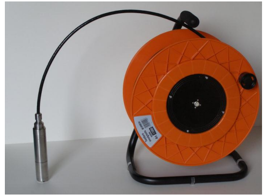
Fig. 3. TPH-485-0,06 transducers with a cable and a coil.
