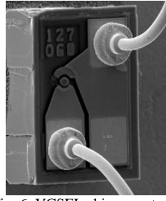
Fig. 6. VCSEL chip mounted on a TO header
