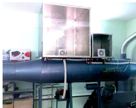
Fig. 2. A fragment of the HAT with a system for sampling and dilution of aerosol.
