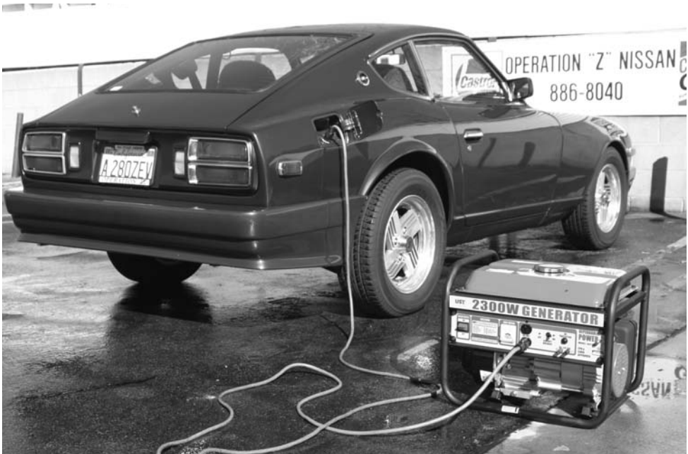
FIGURE 10-31 Operation Z charging connection.
