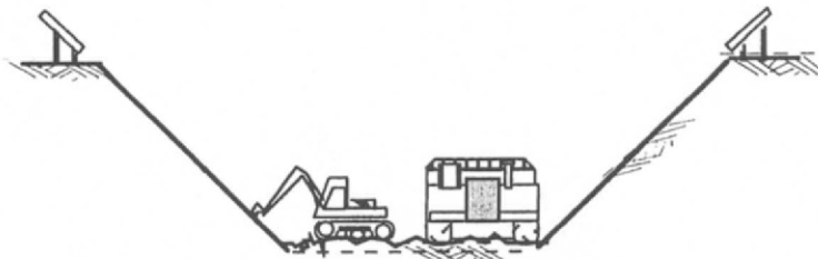
Figure 5.15 Second stage excavation
