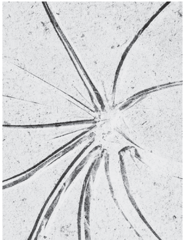
Fig. 58.1 Breakage pattern of annealed glass.
