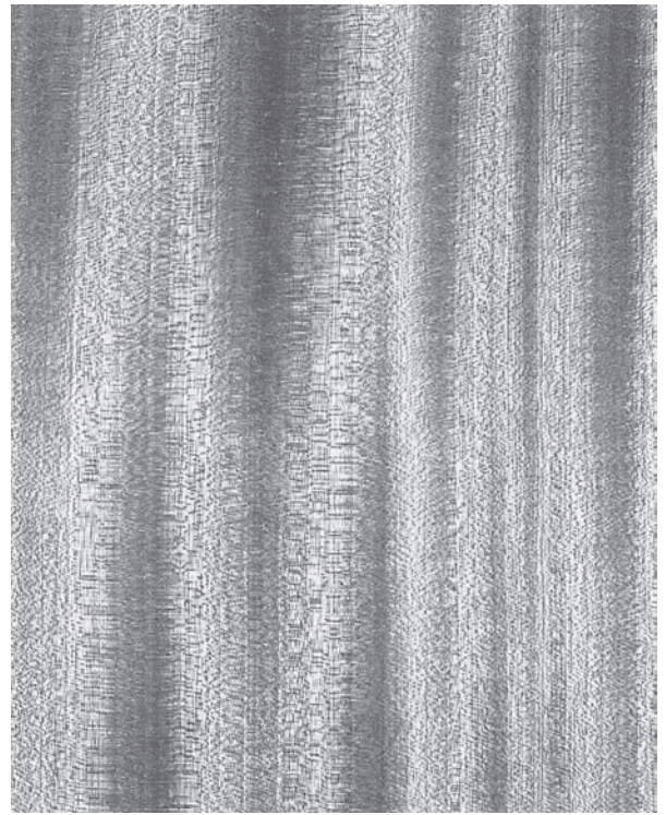
Fig. 52.17 Illustration of ‘ribbon’ or ‘stripe’ figure on the cut longitudinal–radial plane in mahogany timber. The fibres in successive radial zones of the timber are inclined in opposite directions in the longitudinal–tangential plane (© Building Research Establishment).
