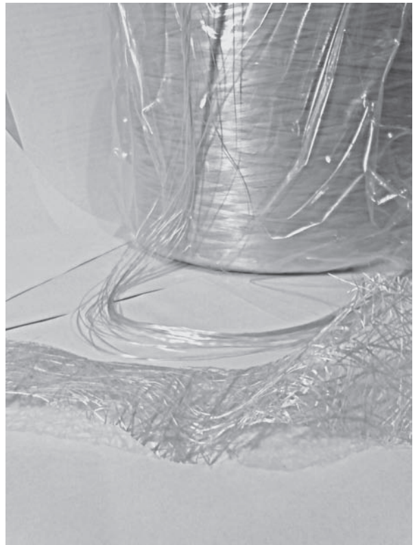
Fig. 45.4 Glass fibres for FRC. Foreground – chopped strand mat. Background – continuous roving for chopping.
