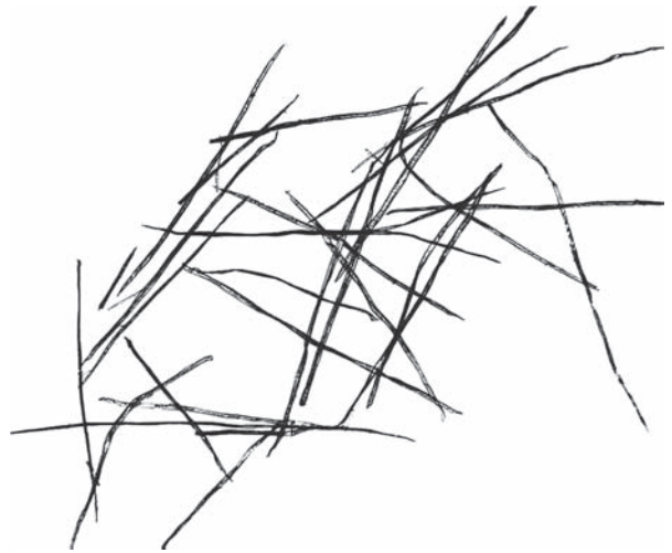
Fig. 52.7 Individual softwood cells (magnification × 12) (© Building Research Establishment).
