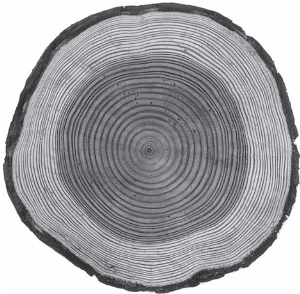
Fig. 52.2 Cross-section through the trunk of a Douglas fir tree showing the annual growth rings, the darker heartwood, the lighter sapwood and the bark (© Building Research Establishment).
