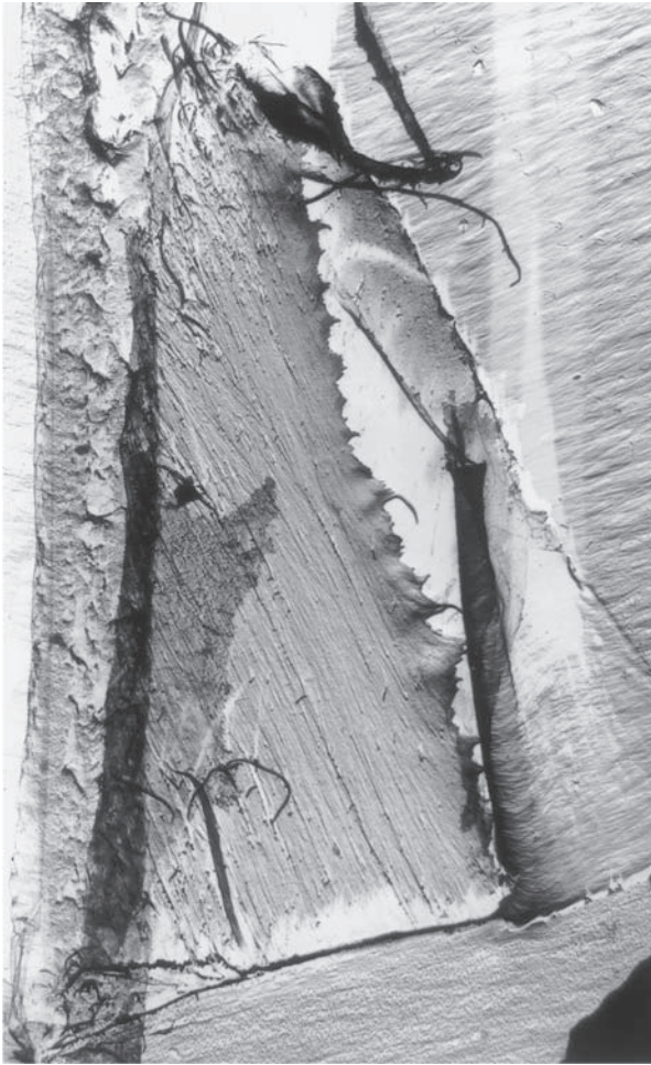
Fig. 52.15 Electron micrograph of the cell wall of Norway spruce timber (Picea abies), showing the parallel and almost vertical microfibrils of an exposed portion of the S_2 layer (© Building Research Establishment).
