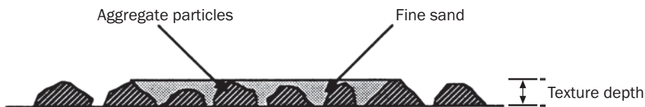
Fig. 27.4 Measurement of macrotexture using the sand patch test.
