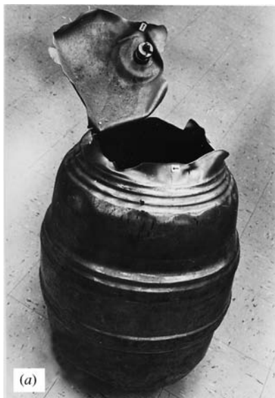
Figure 5.2 Fractured components and devices. (a) Ruptured beer barrel; (b) fractured toilet seat.
