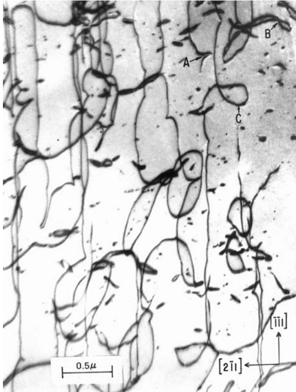
Figure 3.10 Dislocations in silicon-iron thin film. Note dipole trails at A , pinched-off dipoles at B , and independent dislocation movement at the large jog at C . (From Low and Turkalo; 7 reprinted with permission from Low, Acta Met. 10 (1962), Pergamon Press, Elmsford, NY.)
