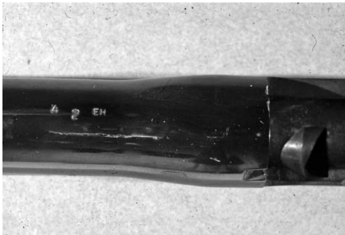
Figure 11.12 Profile of through-thickness \sim 25 -mm-long fatigue crack seen along outer diameter of pre-cracked barrel. Gun barrel subjected to almost 2900 factory rounds of ammunition.
