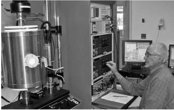
Figure 10.1 Monitoring an environmental fatigue test using computer-controlled instrumentation. (Photo courtesy of J. Keith Donald, Fracture Technology Associates.)
