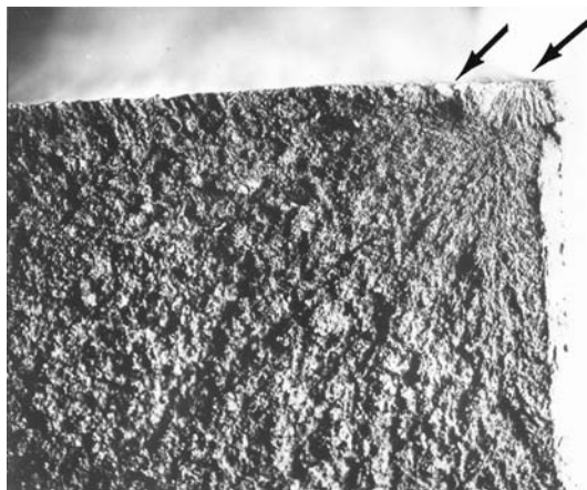
Figure 11.15 Fracture surface of broken eyebar from Point Pleasant Bridge showing two elliptical surface flaws. 22 (Reprinted from Journal of Testing and Evaluation with permission from American Society for Testing and Materials.)
