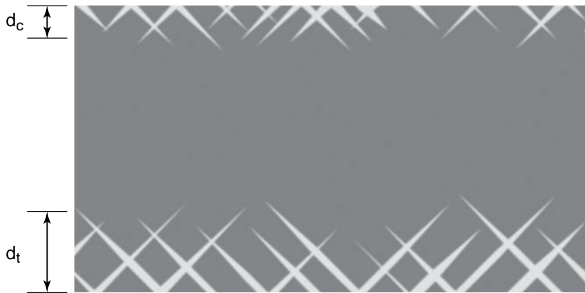
Figure 2.65 Schematic depiction of the cross section of an unplastitized PVC sheet deformed below T_g in 4-point bending. Under cross polarization, shear bands extending from the original surfaces are visible as bright streaks. The approximate shear band depth is marked on the compressive ( d_c ) and tensile ( d_t ) sides of the specimen. The shear band depth is different on the two sides due to pressure-dependent yield behavior.
