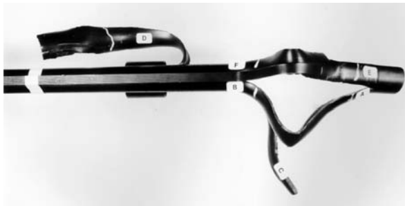
Figure 11.7 Fractured shotgun barrel revealing splayed appearance with fractures occurring essentially along planes parallel to the barrel axis.
