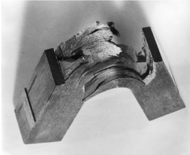
Figure 7.29 Extensive delaminations in ausformed steel with “arrester” orientation. Specimen absorbed 325-J energy. 49 (Copyright American Society for Metals, 1962.)
