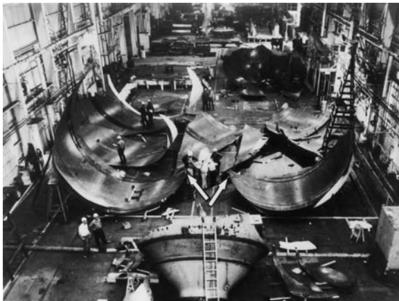
Figure 11.20 Reassembled fragments from ruptured 660-cm rocket motor casing. (From Srawley and Esgar 34 .)
