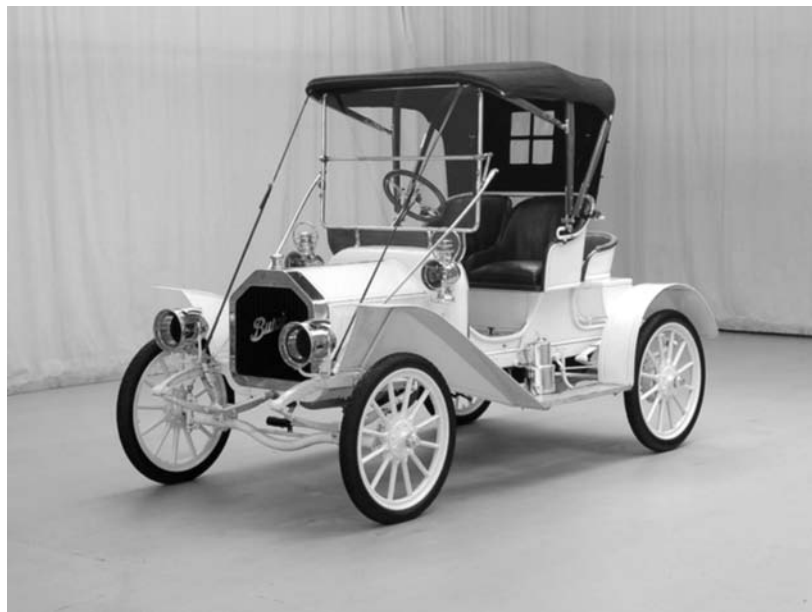
Figure 12.2 Buick Runabout Vehicle, circa 1910. Note the wooden wheel spokes. (M. Hyman and S. Dougan, Hyman Ltd. Classic Cars, St. Louis, MO; photo reproduced with permission from Mark Hyman.)
