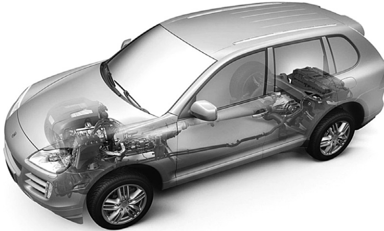
Figure 22.15 Porsche Cayenne Hybrid: system layout.
