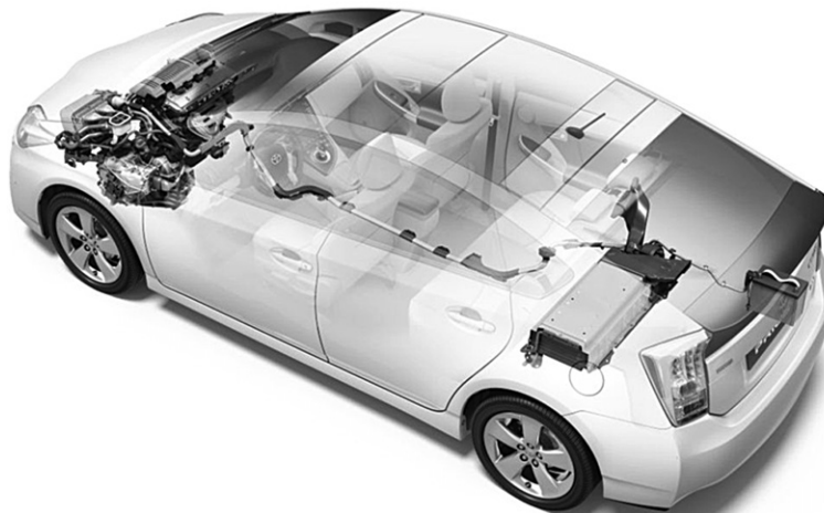
Figure 22.6 Third-generation 2010 Toyota Prius: hybrid system layout.
