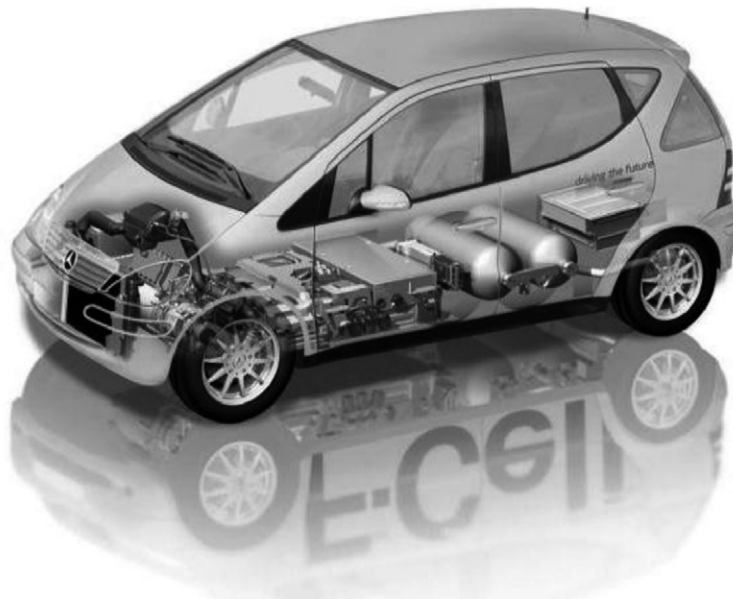
Figure 22.49 Mercedes-Benz B-Class F-Cell: system layout.
