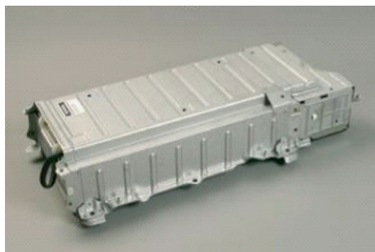
Figure 13.8 Battery system of the Toyota Prius (2006); sealed NiMH, power output: 28 kW, voltage: 201.6V. Expected life based on lab testing: 150,000 miles.
