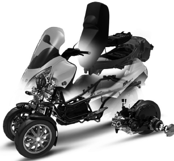
Figure 22.23 Piaggio MP3 HYBRID: system layout.
