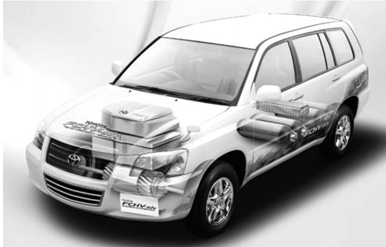
Figure 22.48 Toyota FCHV-adv: system layout.
