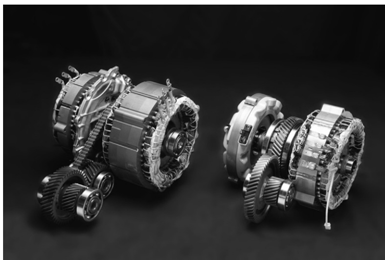
Figure 22.7 Motor-generators: the second-generation Prius transaxle (left) and the new 2010 Prius transaxle (right).
