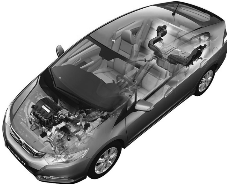
Figure 22.2 2010 Honda Insight: hybrid system layout.
