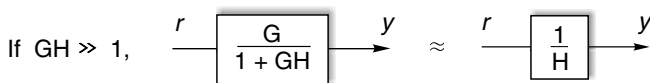
Figure A.5 Simplification of closed-loop system model when loop gain ( GH ) is much greater than 1
