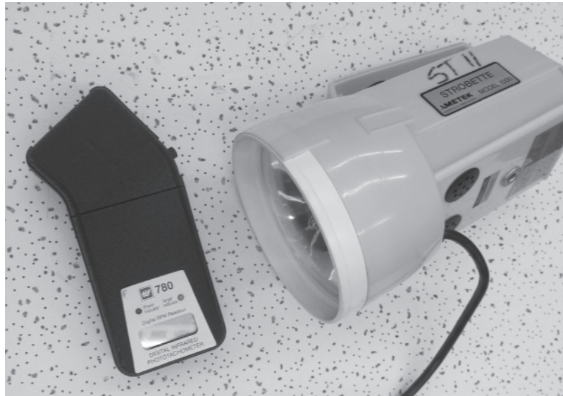
FIGURE 25-5 A strobe tachometer and a photoreflexive tachometer.
