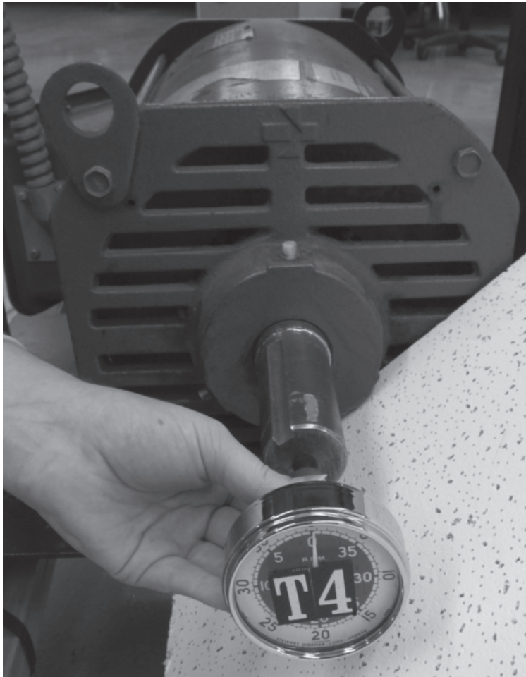
FIGURE 25-6 Mechanical tachometer used to measure shaft RPM.
