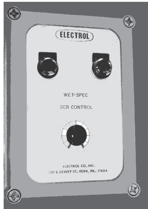
FIGURE 7-7 Control panel for SCR-controlled DC motor drive.
