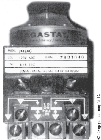
FIGURE 10-10 Mechanical timer uses air (pneumatic) timing.
