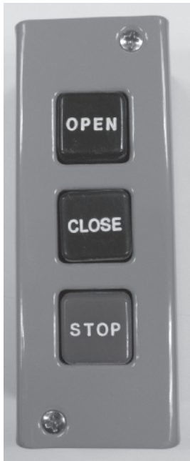
FIGURE 8–1 A forward, reverse, stop pushbutton station.
