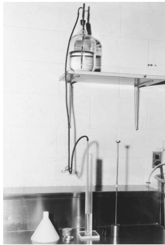
Figure 12 Sand Equivalent Test Apparatus and Procedures: (A) irrigation; (B) Sand Reading; (C) mechanized shaker; (D) graduated cylinder, irrigation tube, weighted foot assembly, and siphon. (From ASTM. With permission.) ©2000 CRC Press LLC
