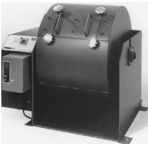
Figure 5 Los Angeles abrasive machine. (Courtesy of ELE International, Inc., Soiltest Products Division, Lake Bluff, IL.)
