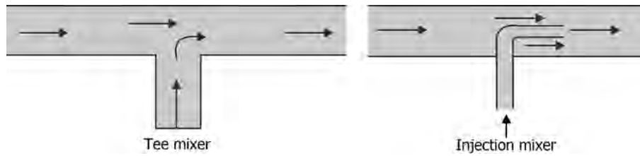
FIGURE 6.16 Tee and injection mixers.
