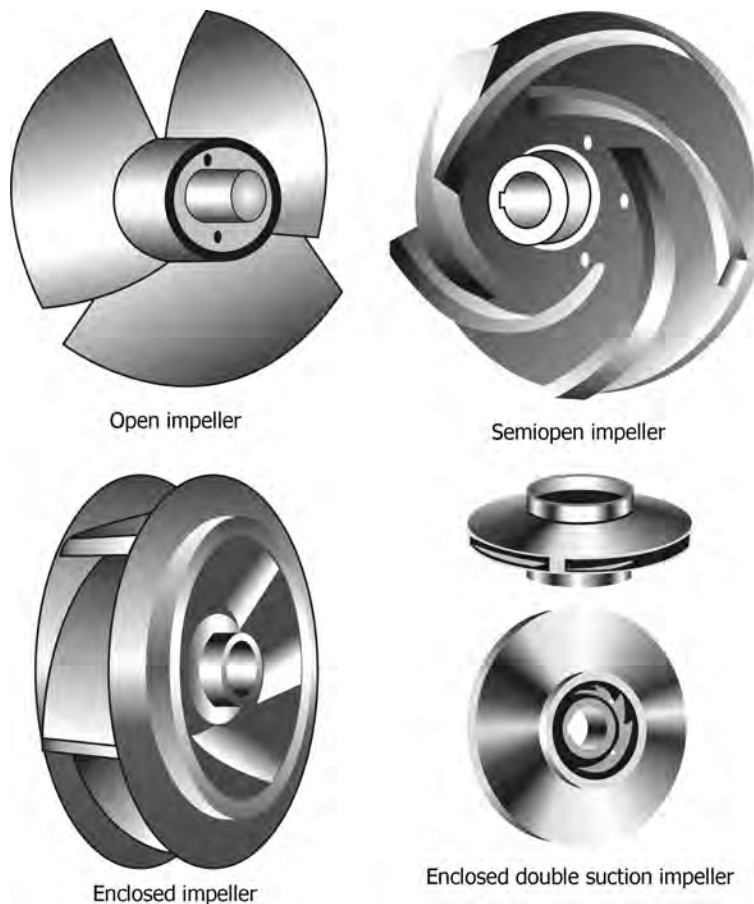
FIGURE 5.5 Open, semiopen, and enclosed impellers.
