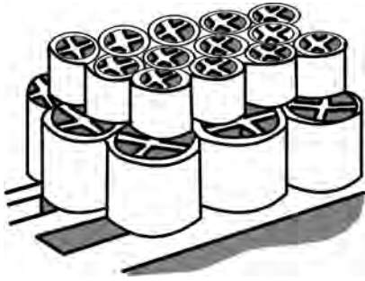
FIGURE 16.23 Stacked packing to support dumped packing.
