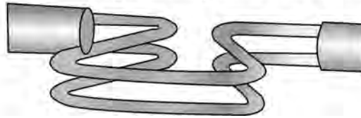
FIGURE 4.30 Double U-tube Coriolis mass flow meter designs.
