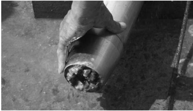
Figure 3.14 Retrieved sand sample retained inside the sampler with the shutter partially closed. (Courtesy of An-Bin Huang, Hsinchu, Taiwan.)
