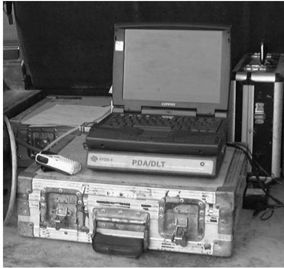
Figure 8.9 Notebook-controlled field pile dynamic testing data logging and analysis system. (Courtesy of An-Bin Huang, Hsinchu, Taiwan.)
