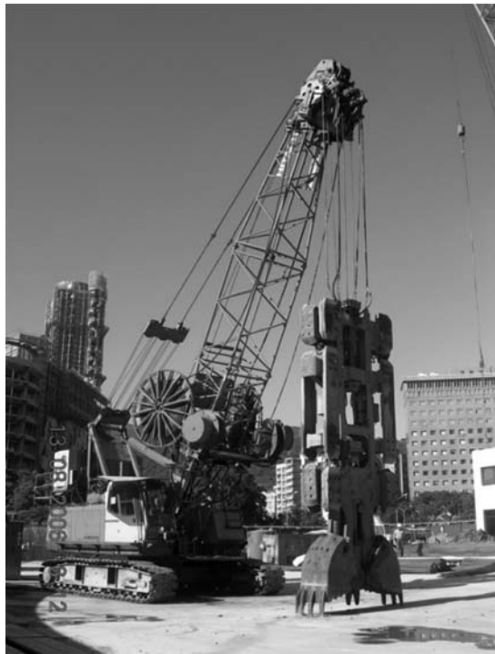
Figure 6.5 Construction crane with a clamshell bucket. (Courtesy of Ground Master Construction Co. Ltd., Taipei, Taiwan.)
