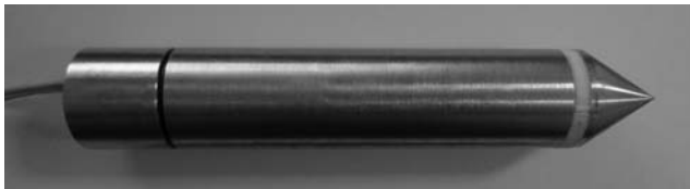
Figure 3.28 A piezocone with porous element at u_2 position. (Courtesy of An-Bin Huang, Hsinchu, Taiwan.)
