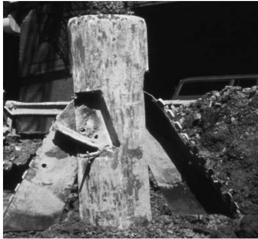
Figure 8.30 A belling bucket with unfolded arms. (Courtesy of An-Bin Huang, Hsinchu, Taiwan.)
