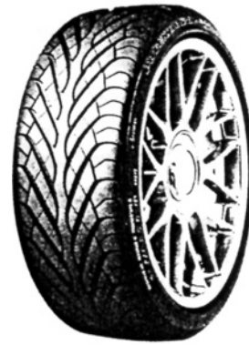
Figure 22.14 Bridgestone ultra high-performance sports tyre with super slant tread pattern ( Bridgestone/Firestone )
