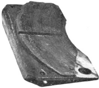
Figure 27.29 Disc pad neglect in service ( Ferodo )
