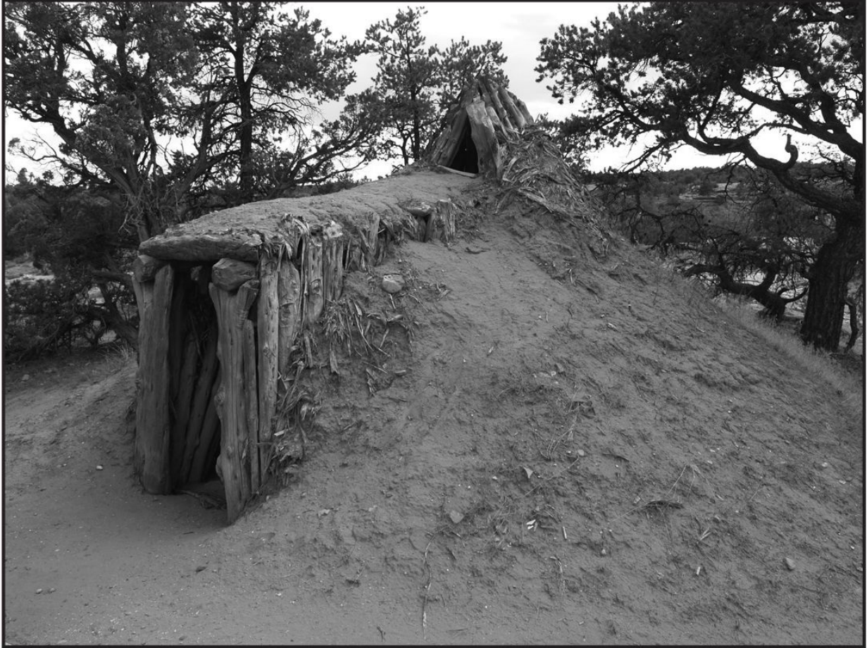
A traditional Navajo hogan, framed with timbers and covered with dirt.
