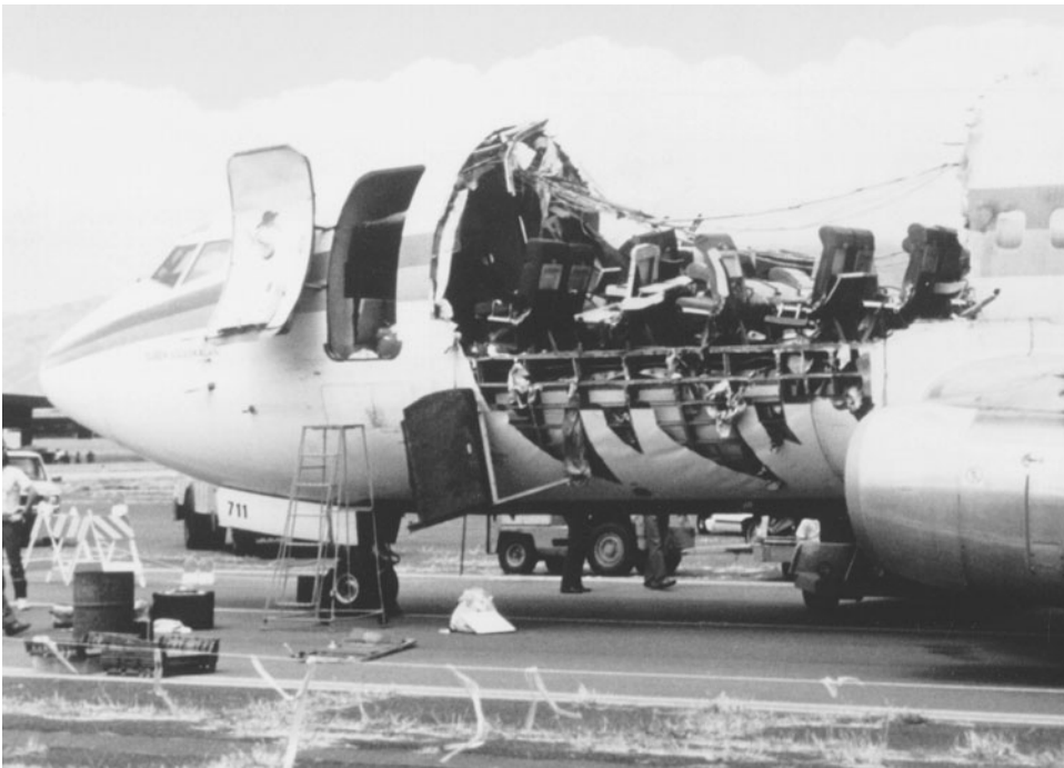
Figure 1.11 Fuselage failure in a passenger jet that occurred in 1988. (Photo courtesy of J. F. Wildey II, National Transportation Safety Board, Washington, DC; see [NTSB 89] for more detail.)
