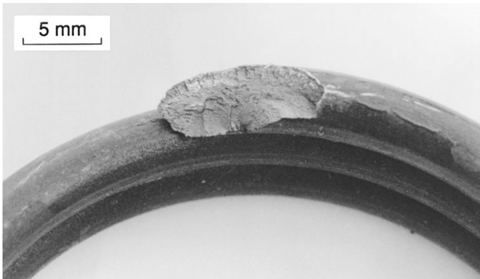
Figure 1.9 Fatigue failure of a garage door spring that occurred after 15 years of service. (Photo by R. A. Simonds; sample contributed by R. S. Alvarez, Blacksburg, VA.)
