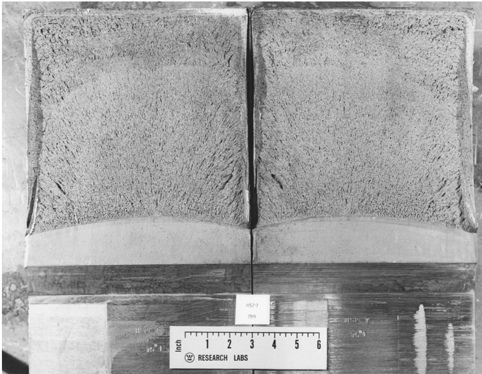
Figure 8.30 Fracture surfaces from a K_{Ic} test on A533B steel that used a compact specimen of dimensions t = 25 , b = 51 cm. (Photo courtesy of E. T. Wessel, Haines City, FL; used with permission of Westinghouse Electric Corp.)
