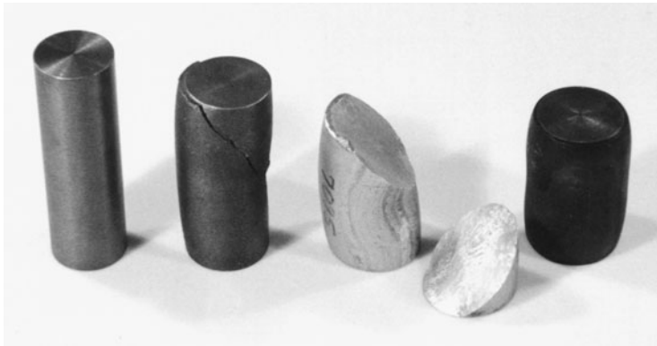
Figure 4.23 Compression specimens of metals (left to right): untested specimen, and tested specimens of gray cast iron, aluminum alloy 7075-T651, and hot-rolled AISI 1020 steel. Diameters before testing were approximately 25 mm, and lengths were 76 mm. (Photo by R. A. Simonds.)
