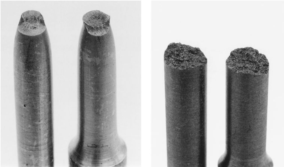
Figure 4.13 Fractures from tension tests on 9 mm diameter specimens of hot-rolled AISI 1020 steel (left) and gray cast iron (right). (Photos by R. A. Simonds.)
