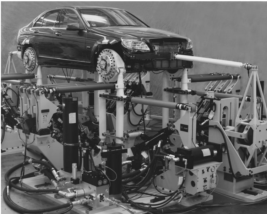
Figure 1.13 Road simulation test of an automobile, with loads applied at all four wheels and the bumper mounts. (Photo courtesy of MTS Systems Corp., Eden Prairie, MN.)
