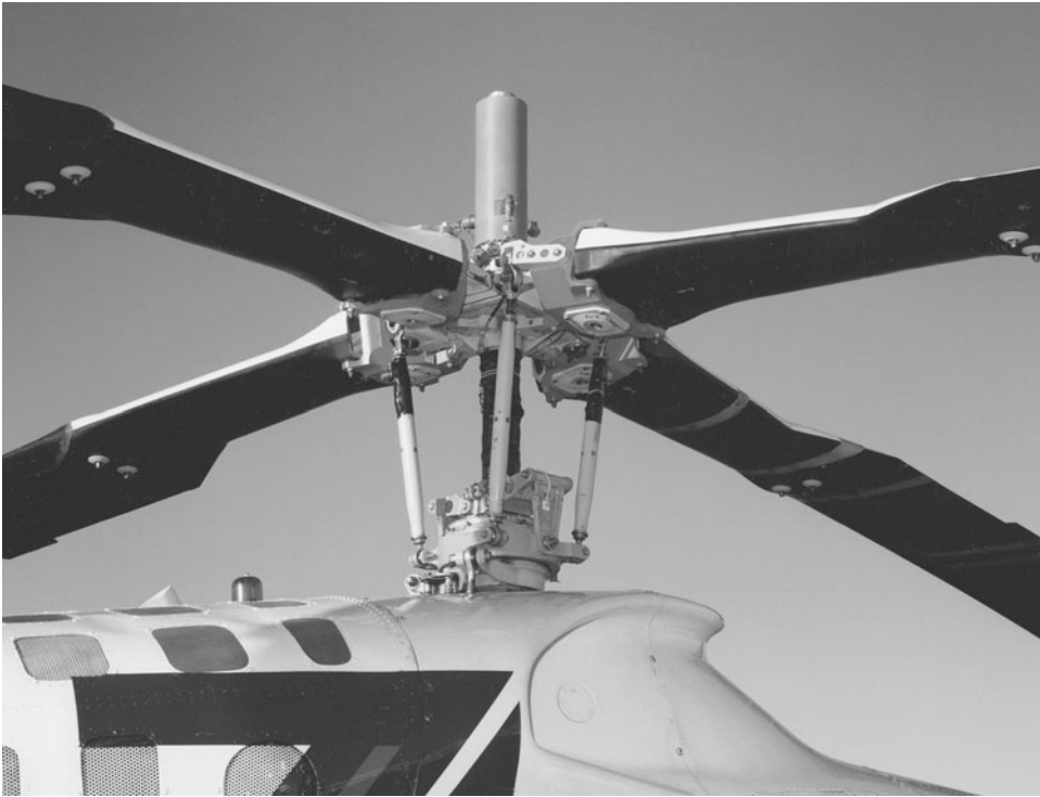
Figure 1.10 Main mast region of a helicopter, showing inboard ends of blades, their attachment, and the linkages and mechanism that control the pitch angles of the rotating blades. The cylinder above the rotors is not ordinarily present, but is part of instrumentation used to monitor strains in the rotor blades for experimental purposes. (Photo courtesy of Bell Helicopter Textron, Inc., Ft. Worth, TX.)
