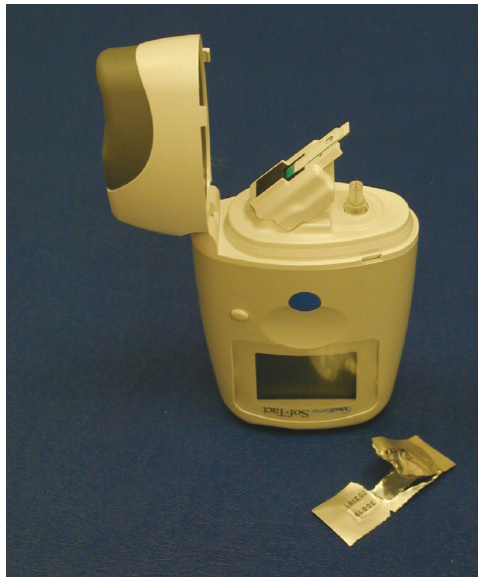
FIGURE 23.3 Sof-Tact meter with cover opened to load test strip and lancet. Test strip is inserted into an electrical connector. The hole in the opposite end of the test strip allows the lancet to pass through. The white cylindrical lancet is loaded into the lancet tip holder in the housing. To perform a test, the cover is closed, the gray area of the cover placed against the skin and the front button depressed.
