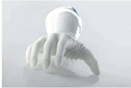
FIGURE 42.6 The Michelangelo Bionic Hand. (Otto Bock Healthcare, GmbH, Duderstadt, Germany.)
