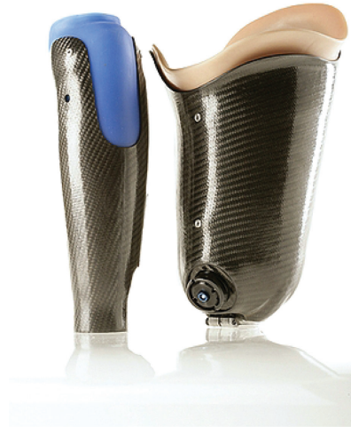
FIGURE 42.4 Otto Bock SiOCX socket system (Otto Bock Healthcare, GmbH, Duderstadt, Germany). The socket consists of an inner made of HTV silicone that connects to the outer composite socket using a mechanical screw interface.
