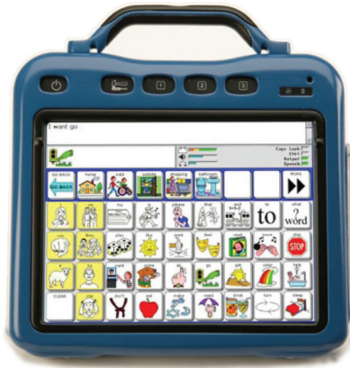
FIGURE 47.2 Example of a touch screen AAC user interface with a language software application with 45 locations that provides all three language representation methods.
