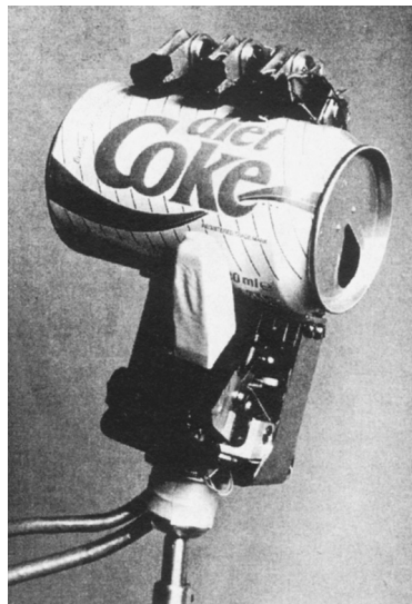
FIGURE 44.10 Southampton hand prosthesis with four degrees of freedom in a power grip. An optical/acoustic sensor is mounted on the thumb. (Reprinted from Chappell, P.H. and Kyberd, P.J. 1991. J. Biomed. Eng. 13: 363.)
