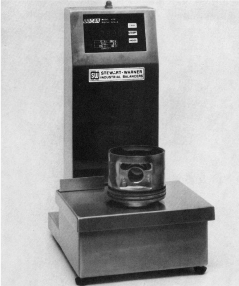
8-79 Balancing begins with match-weighing piston assemblies.
