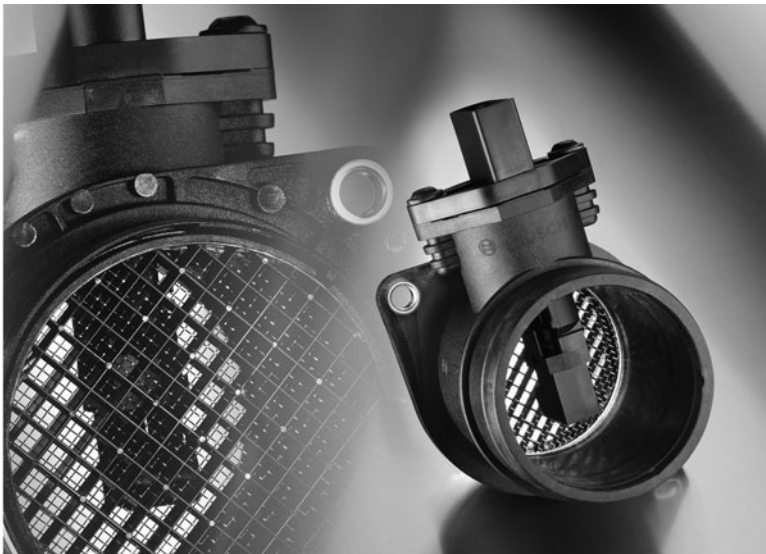
6-10 The hot-film air mass sensor measures the amount of current needed to maintain its sensing element, one side of which is cooled by incoming air, at a predetermined temperature. Courtesy Bosch
