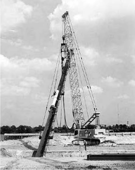
Figure 3.4 Liebherr LRH 400 48 m long swinging leader on HS 885 HD crane (courtesy Liebherr Great Britain Ltd).
