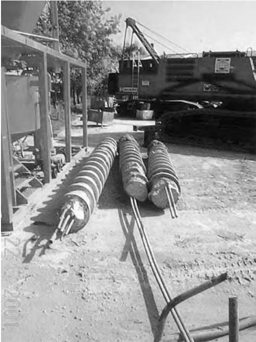
Figure 2.29 (a) The ScrewSol tapered auger and tight-fit follower tube (b) Cleaned-off section of an excavated ScrewSol pile.
