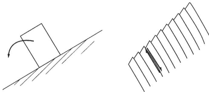
Figure 17.9 Direct and flexural modes of toppling instability.
