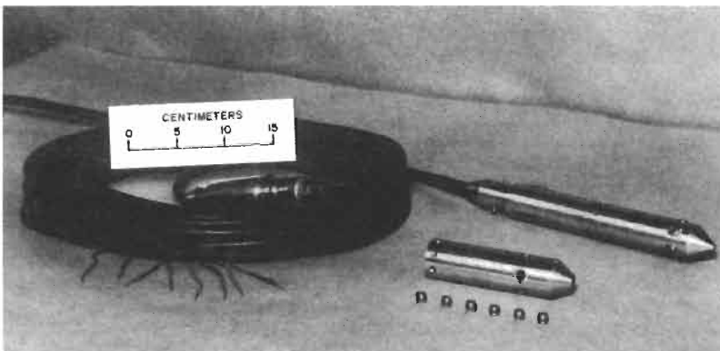
Figure 4.7 The USBM borehole deformation gauge.
