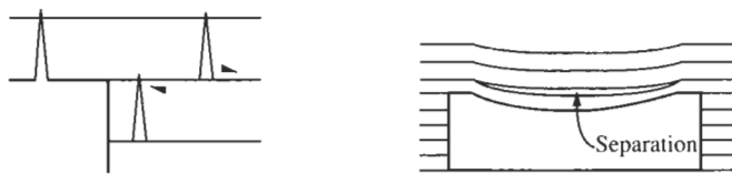
Figure 19.21 Composite instability around excavations in stratified rock.
