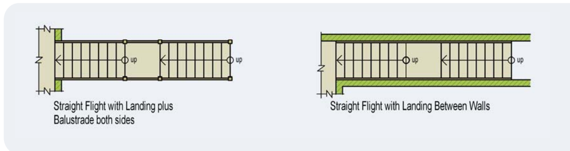
Figure 1.3: Straight stairs with landing.
