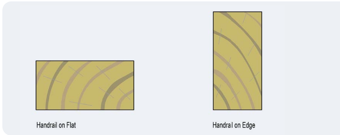
Figure 6.2: Handrails – on flat and on edge.
