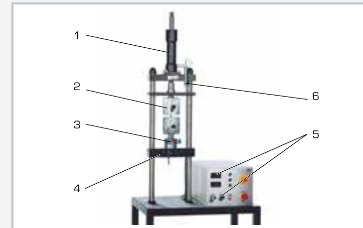
1 hydraulic cylinder for generating tensile and compressive forces, 2 operating area with the accessory WP 310.05, 3 force sensor, 4 adjustable height lower cross-member with lock, 5 displays and controls, 6 displacement sensor
