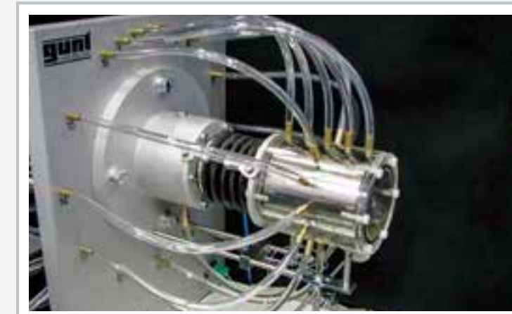
Detailed view of the TM 280 journal bearing unit
