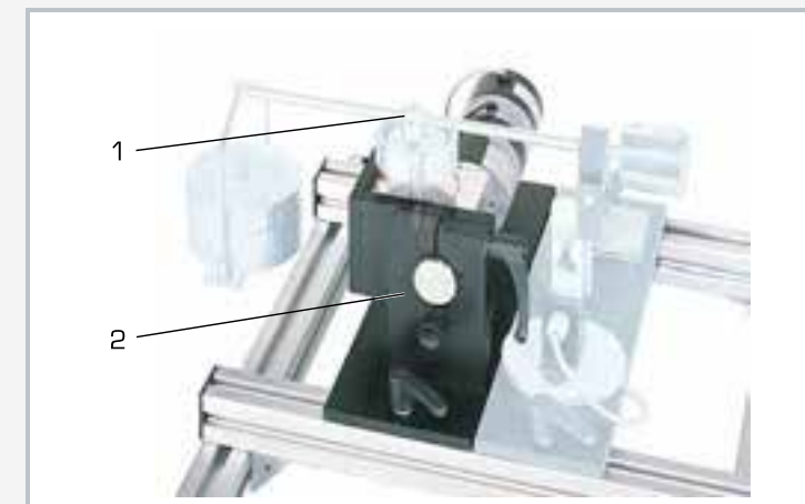
1 TM 260.03 experimental unit studies a tribological system, consisting of a pin and disk, which slide against each other, 2 TM 260 drive unit
