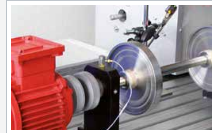
Application of the sensors: acceleration sensor on the black bearing support, speed sensor with holder
