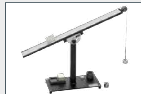
TM 225 Friction on the inclined plane
