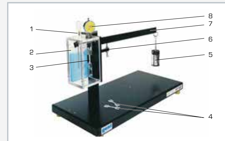
1 thermometer for temperature-controlled box, 2 storage element for cooling the specimen, 3 clamped specimen, 4 specimens, 5 weight, 6 adjustable stop for the lever, 7 lever, 8 dial gauge
