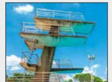
Bending stress of a cantilever beam using the example of a diving board
