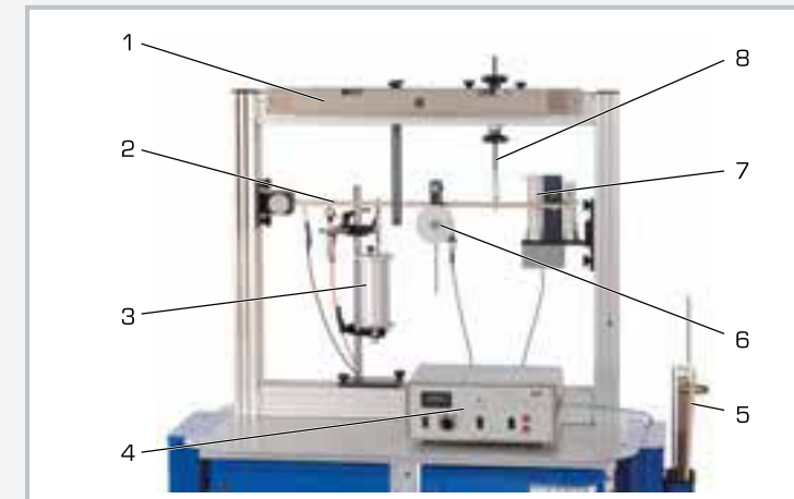
1 pendulum bearing, 2 bar-type oscillator, 3 container for oil damper, 4 control unit for imbalance exciter, 5 storage for additional pendulums, 6 imbalance exciter, 7 drum recorder, 8 spring
