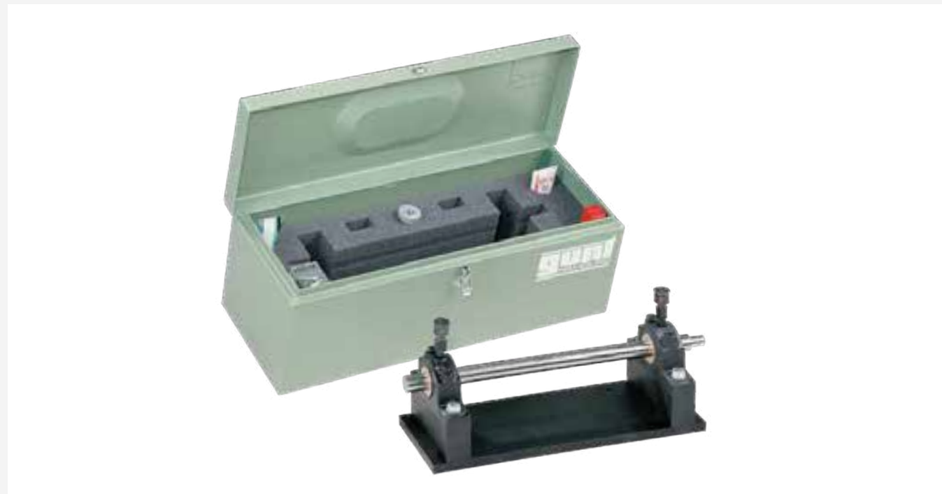
The illustration shows the tool box with the assembly kit and, in the foreground, the fully assembled journal bearing
