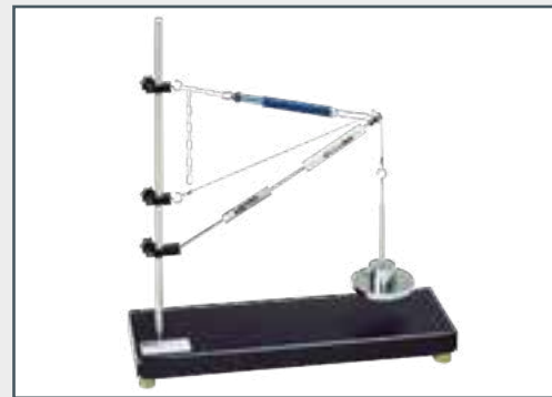
TM 115 Forces in a crane jib
