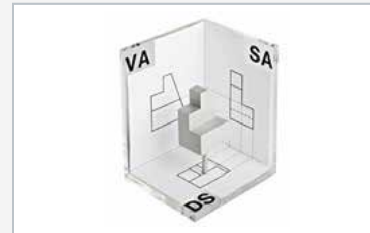
Room corner made of three Plexiglas planes with inlaid drawing and a prismatic model
