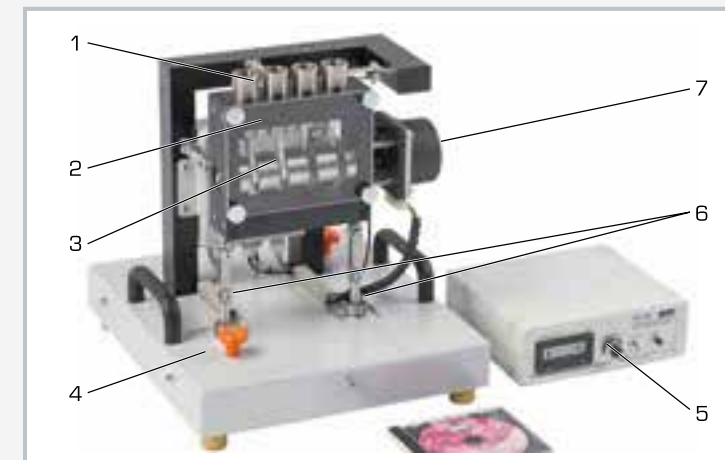
1 piston, 2 cylinder, 3 crankshaft, 4 foundation plate, 5 display and control unit, 6 force sensor, 7 drive motor
