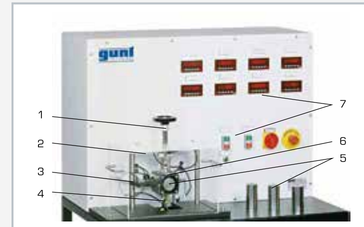
1 handwheel for load, 2 transparent protective cover, 3 oil pressure line, 4 force sensor for frictional moment, 5 shaft, 6 bearing housing with inductive displacement sensors, 7 displays and controls
