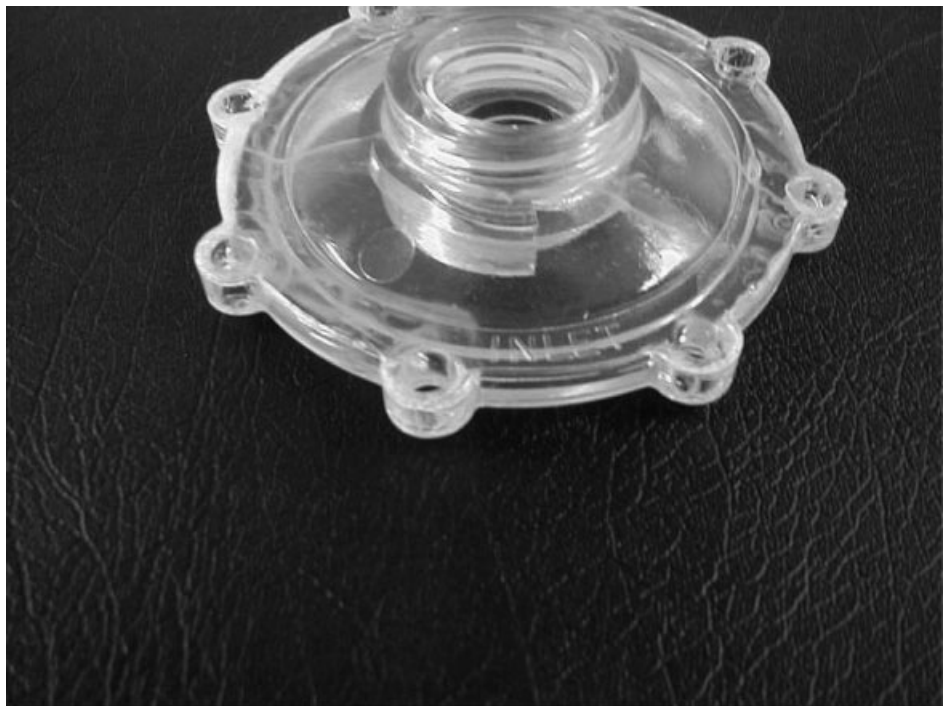
Figure 10 Result of solvent attack in terms of crazing and cracking around highly stressed mounting holes.
