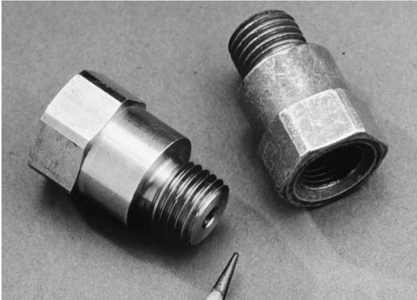
Figure 10 Hose fitting, a typical automatic screw machine part made in alloy C36000 (left) and free-cutting brass and 12L14 leaded steel (right). The brass version typically provides lower finished cost.
