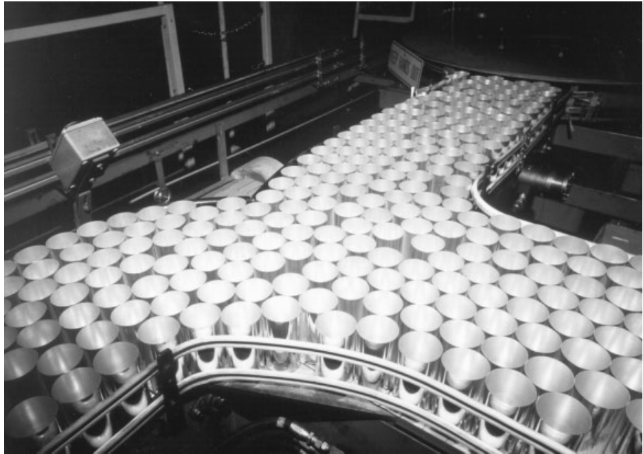
Figure 7 Bodies of most beverage cans are alloy 3004, the ends are 5182, making it the largest volume alloy combination in the industry.
