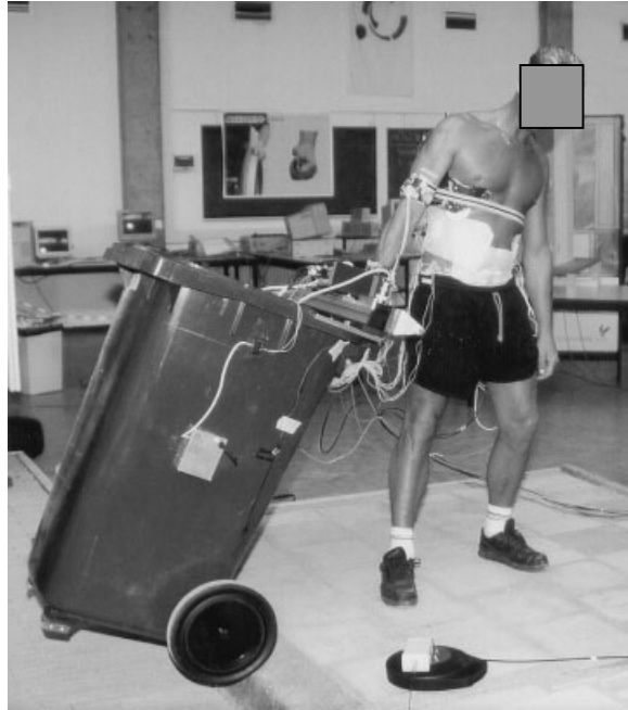
Figure 3 Refuse collector during data collection for estimation of mechanical workload in pulling refuse container up pavement.
