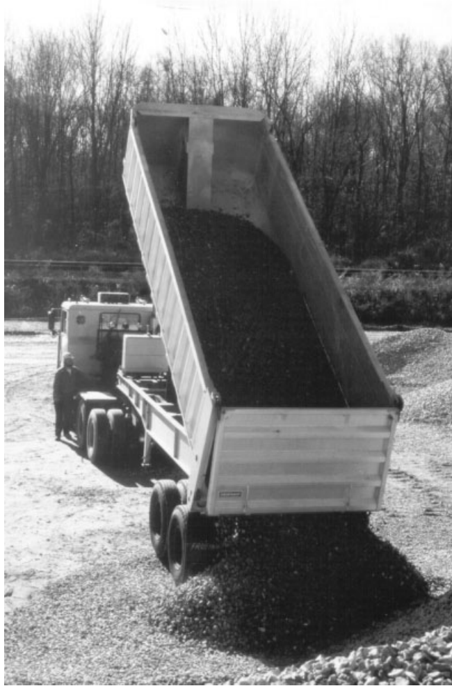
Figure 4 Heavy dump and tank trucks and trailer trucks employ high-strength 2xxx or 6xxx extrusions for their structural members and tough 5xxx alloy sheet and plate for their load-carrying components.
