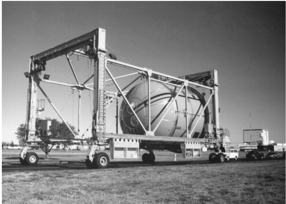
Figure 5 Fuel tanks and booster rockets such as those of the Space Shuttle are 2xxx alloys, originally 2219 and 2419, now Al–Li “Weldalite” alloy 2195.
