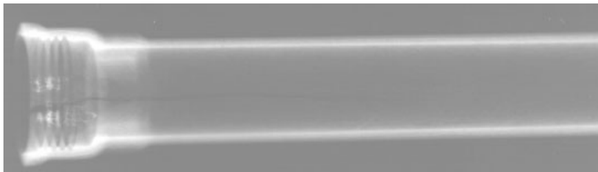
Figure 7 A radiograph of a crack in end of aluminum tubing.
