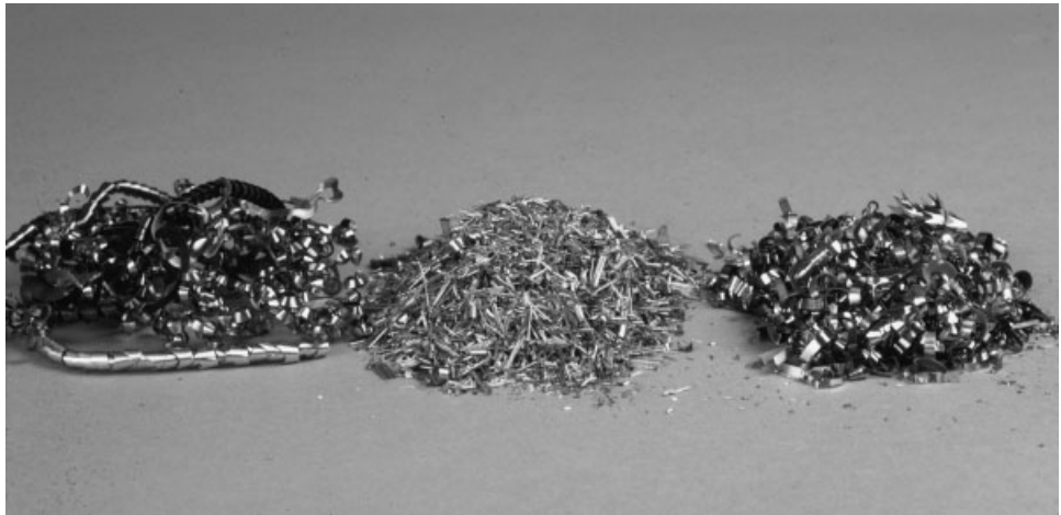
Figure 2 Three types of machining chips produced by copper and copper alloys: type I (free-cutting) chips, center; type II (short curly chips), right; type III (long stringy chips), left.
