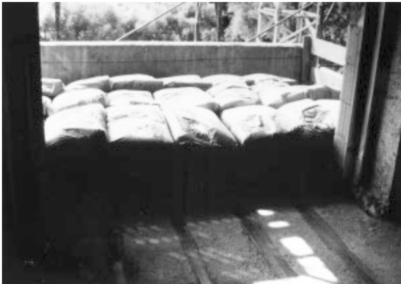
Figure 11.36 Load testing of balcony at Loano.
