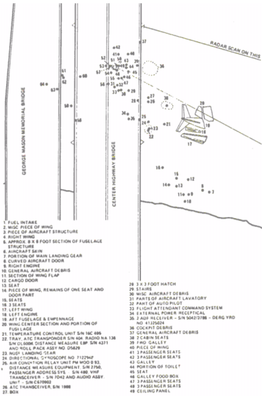
Figure 7.14 Wreckage location chart, reconstructed from underwater radar scan and manual plotting.
