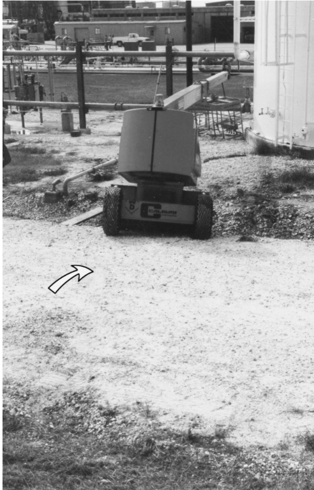
Figure 4.3 The front wheels of this aerial platform moved into a ditch at an oblique angle to the roadway. The arrow indicates a scuff mark left by one of the tires before the unit slid into the ditch.
