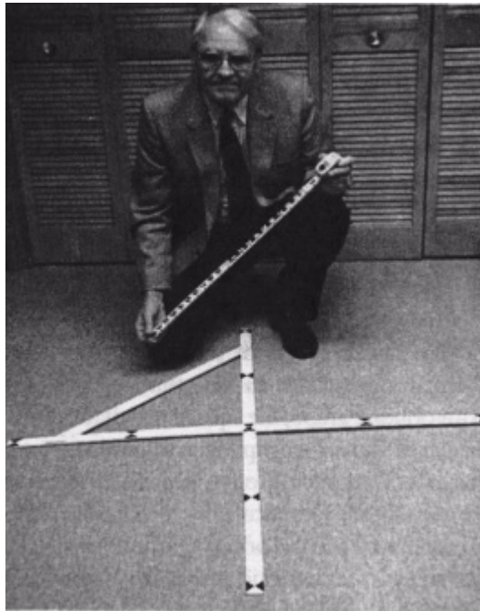
Figure 11.4 The author holds a linear scale graduated in hundredths of a foot. A folding, 4-foot, two-dimensional scale is shown in the foreground.
