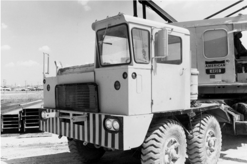
Figure 4.12 This crane cab was the subject of critique after an electric shock injury to a ground worker when a boom cable touched an electric transmission wire. Note that the boom forward windshield tilts forward.
