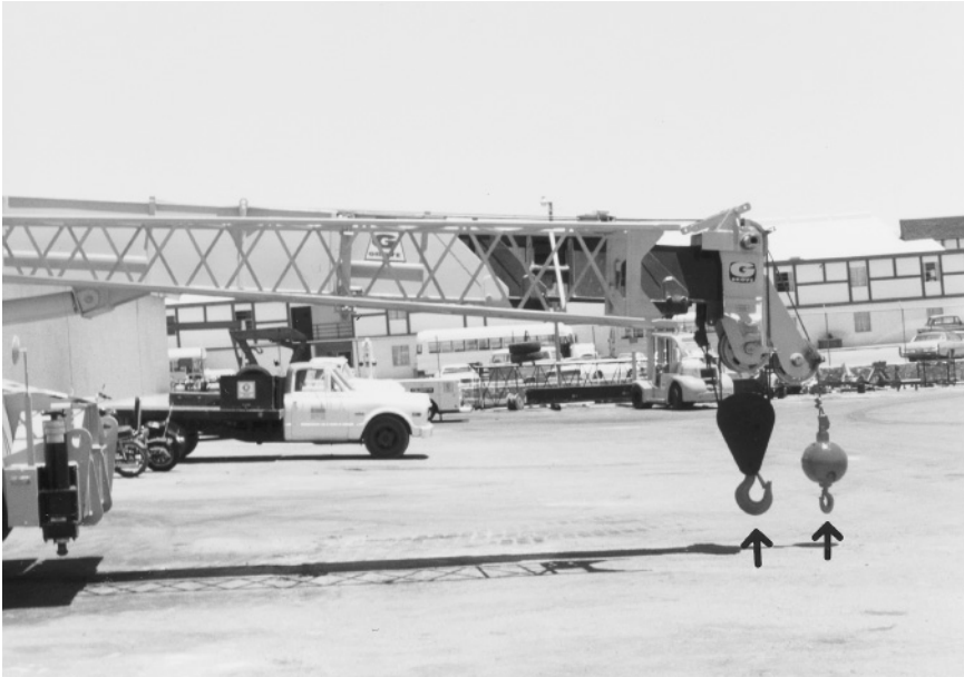
Figure 4.19 The two cable and block systems that were in use on the extendible boom. Two blocking occurs when the boom is maneuvered in such a way that the boom cable becomes too short and attempts to pull the block into the boom.
