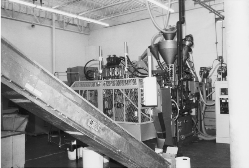
Figure 4.4 Blowmolder and its barrier guards. An operator had obviated the guards by standing on an upside-down bucket and reaching over the top of the guard, placing his hands in the area of the molding process.
