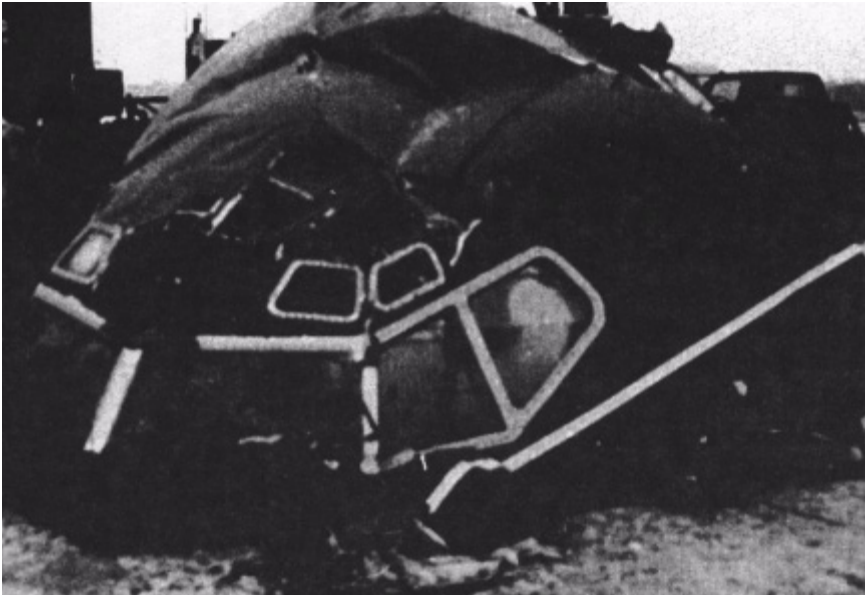
Figure 7.15 Section of forward top of fuselage (cockpit area) after recovery. (Courtesy NTSB.)
