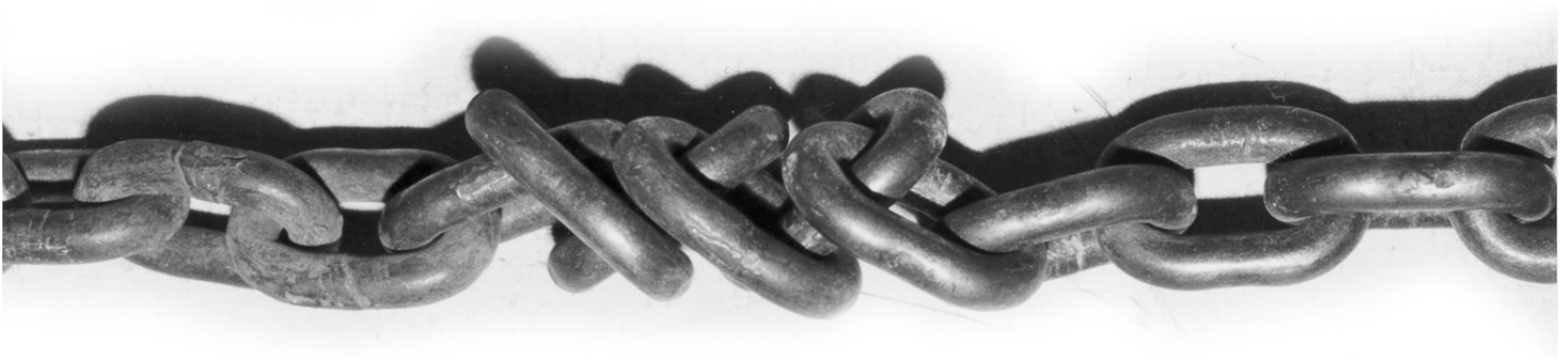
Figure 4.2 Section of the chain used on the chain fall hoist. The chain rotated and doubled up. A metal chain is much weaker in this mode and is vulnerable to premature failure.
