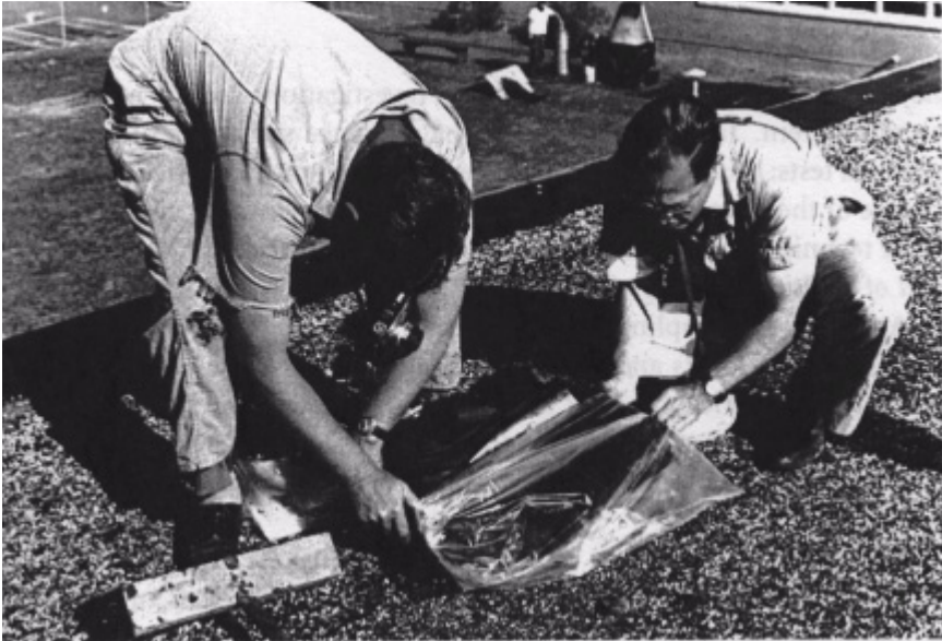
Figure 8.10 Field samples must be carefully documented, labeled, and packed for shipping to the laboratory.
